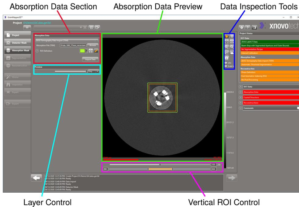
(TXM) has been specified, the **Absorption Data Preview** displays the horizontal slice of the absorption data centered in the aperture FOV. The **orange** rectangle on the preview indicates the horizontal aperture FOV, while the ROI Definition is shown in **green**.
