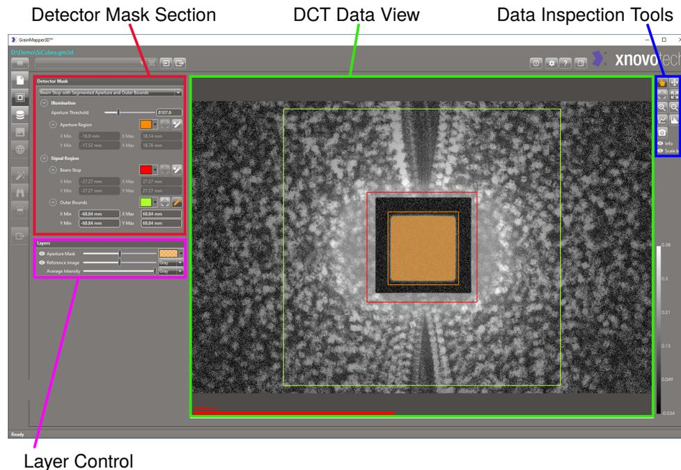
The **DCT Data View** now also shows the **Reference Image** if present. The visual appearance can be adjusted using the **Layers** control as described in Table 5.
