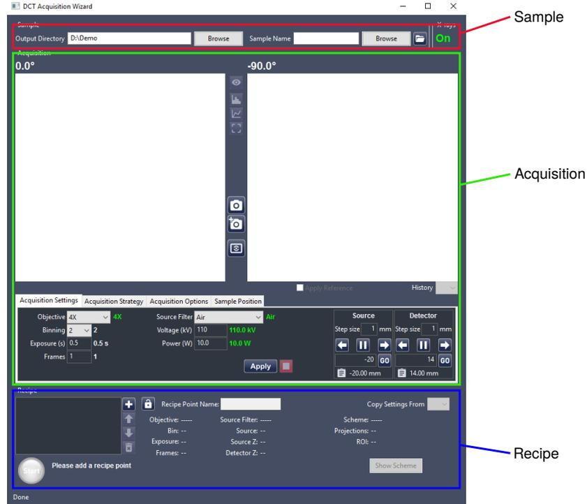
The *look and feel* of the DCT Acquisition Wizard is similar to Scout-and-Scan, and the user should be able to recognize many of the controls, for instance in the **Acquisition Settings**, **Sample Position** and **Recipe** sections.
