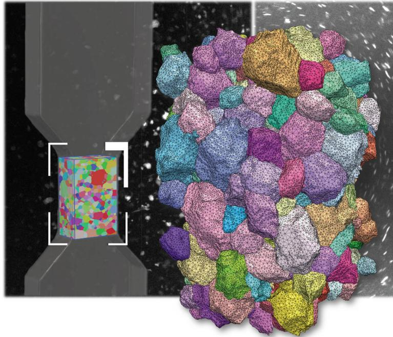
While the *conventional* DCT scan performed using Scout-and-Scan is applicable when the *sample region of interest* (ROI) fits in the *beam field of view* (FOV), the DCT Acquisition Wizard allows for collecting DCT data with three new *advanced* acquisition strategies for samples where the ROI does not fit in the FOV.
