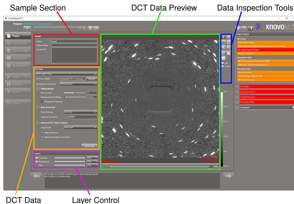
**Background Correction** The former DCT data import options have been moved into the **Rolling Median** background correction method and a new **Iterative Background** correction method has been added. [Table 1](#) details the new controls for **Background Correction** of the Diffraction Contrast Patterns (DCPs).
