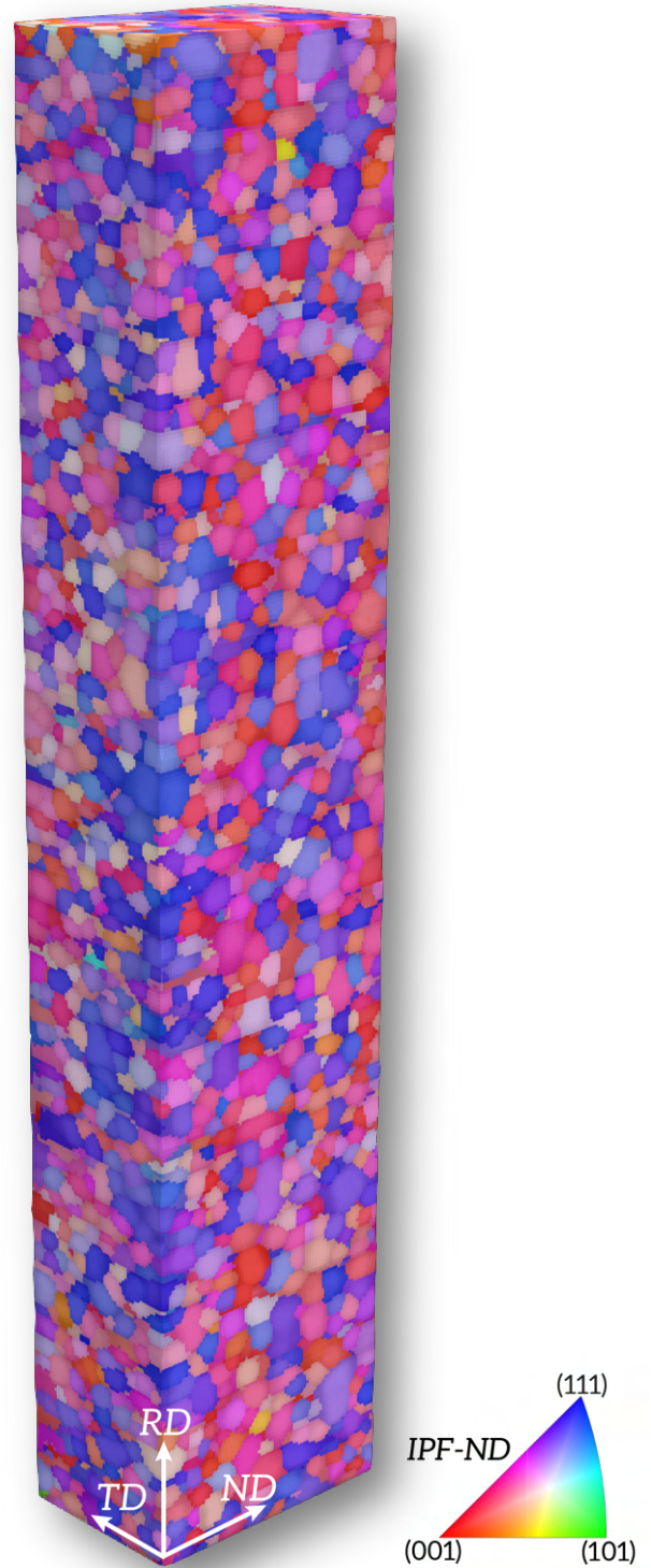
Figure: 3D grain map of the mapped sample volume, colored by IPF-ND with respect to sample normal direction. Dimensions: 2 mm (RD), 0.4 mm (TD) and 0.4mm (ND).
