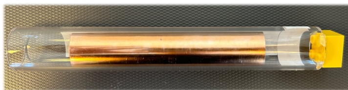
Photo: Cu coil sample protected in quartz tube. The sample is scanned as presented in the photo, mounted using a LEGO brick.
