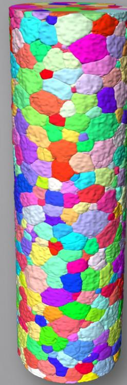
Al alloy, cubic,  $\text{\O} \sim 1.4 \times 5.5$  mm
