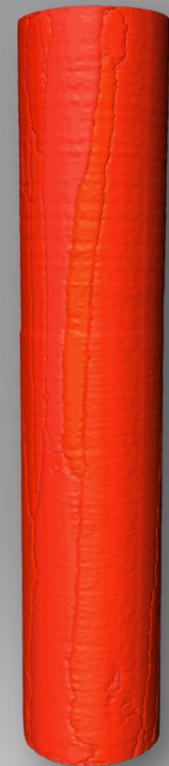
Ni superalloy, cubic,  $\text{\O} \sim 2 \times 9$  mm
